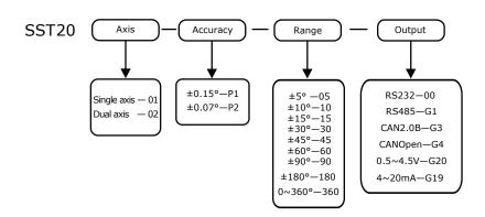
For example: if order a dual-axis SST20 inclinometer, range  $\pm 60^{\circ}$ ,  $\pm 0.07^{\circ}$  accuracy, output CAN2.0B, the model should be chosen as : SST20-02-P2-60-G3
