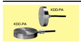
The KDC-PA and KDD-PA are anticorrosion stainless-steel soil pressure gauges each 100 mm in outside diameter. They are used to measure the pressure in soil in ocean or coastal civil engineering structures and to measure the dynamic pressure of waves. With the KDC-PA, the Input/Output cable comes from the side of body. With the KDD-PA, the cable comes from the back of body. Protection ratings: IP 68 equivalent
