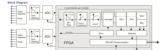
Arithmetic and signal conditioning: min, max, +, -, \*, /, integ. etc.
