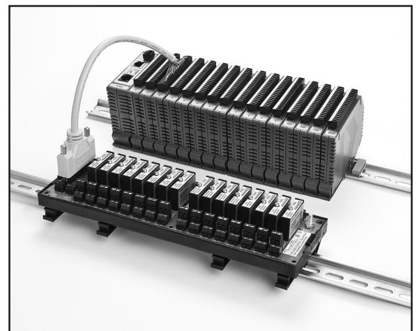
Figure 3: Cable Interfacing 8B Backpanel to MAQ20-VSN Module
