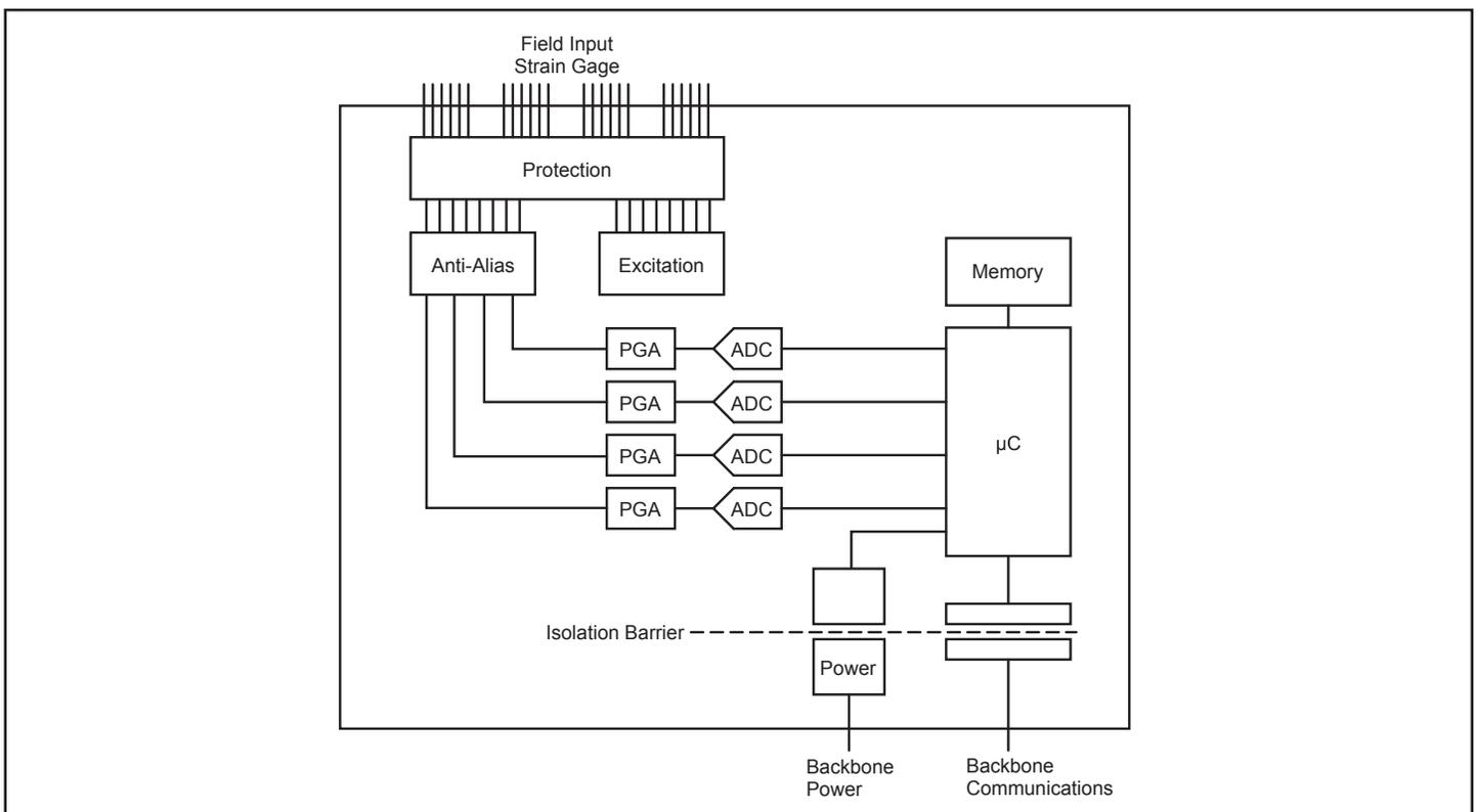
Figure 1: MAQ20 Strain Gage Input Module Block Diagram
