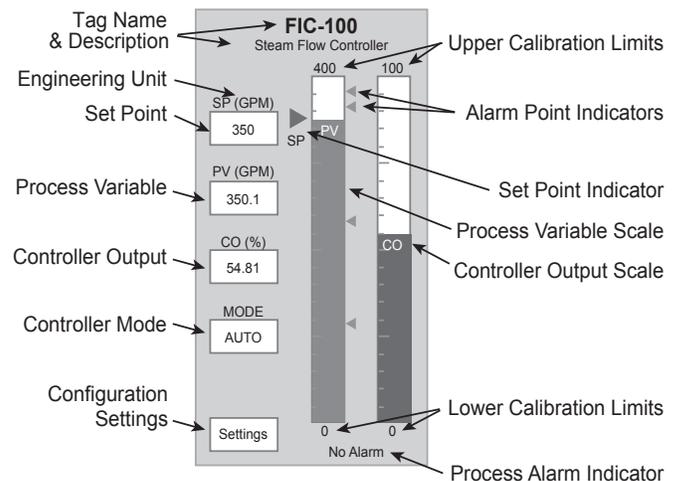
Figure 2: PID Faceplate in ReDAQ Shape Software
