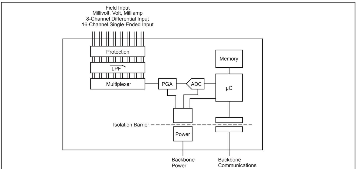
Figure 1: MAQ20 Voltage & Current Input Module Block Diagram
