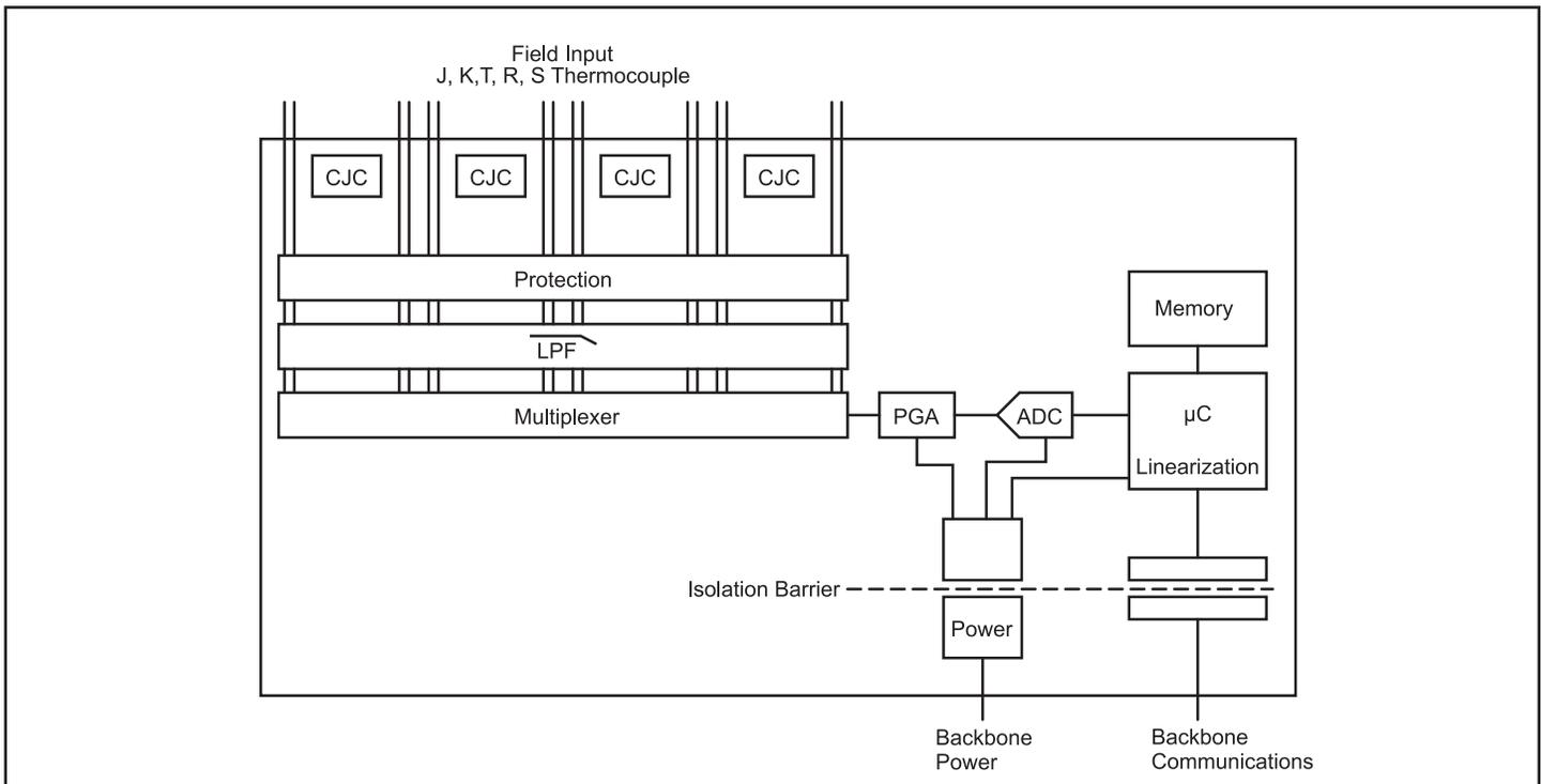
Figure 1: MAQ20 Thermocouple Input Module Block Diagram
