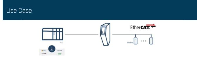
The communicator can be used wherever there is a need to transfer data between control systems using different industrial protocols.
