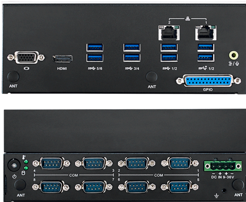
Figure 2.2 ARK-3531 Front and Rear I/O Connector Diagram
