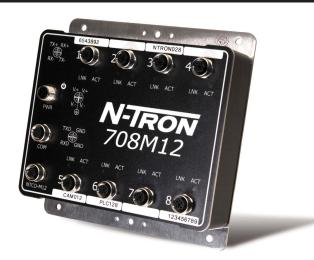
**DHCP** - DHCP Server/Client automates the assignment of IP addresses. DHCP Option 82 assures that if a device on a specific port is replaced, the replacement receives the same IP address as the original device.
