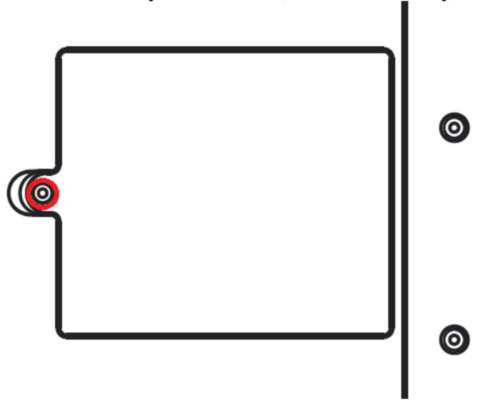
3. Once the HDD bay cover has been removed, unscrew the 4x screws on the HDD bracket highlighted below. Then slide the HDD out to unplug and lift to remove.
