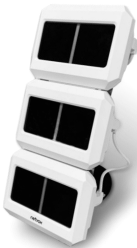
Three DSC100C connected in parallel
