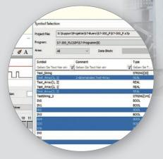
Importing the variables All variables from the symbolics of the PLC project are imported into the measurement program and are immediately available for any type of analysis.
