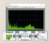
Create an oscilloscope with FFT signal evaluation using only **three modules**.
