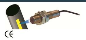
**IRS (Infrared Sensor):** Ideal sensor for working up to 0.5" (12mm) from high speed equipment or other applications providing only contrasting light and dark surfaces or beam interruption by solid objects as small as 0.30" (1mm).
