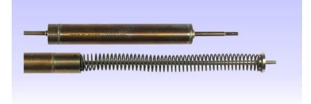
These transducers are for displacement / position measurement. They make an accurate position measurement of the movement of the armature (the sliding part) relative to the body of the displacement transducer.
