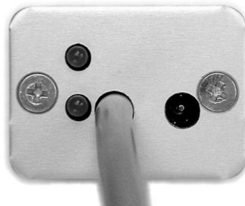
Fig. 34 – indicators, cable and power supply connector
