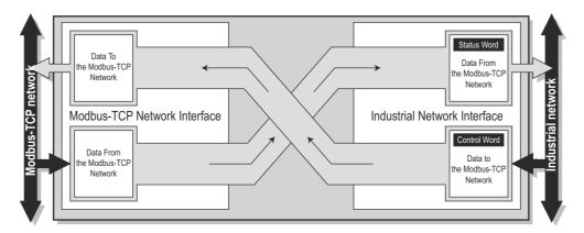
Each buffer holds a maximum of 256 bytes of data. The first two I/O mapped bytes in either direction can be dedicated for control/status information, and another eight bytes of data coming from Network 2 can feature a live list.
