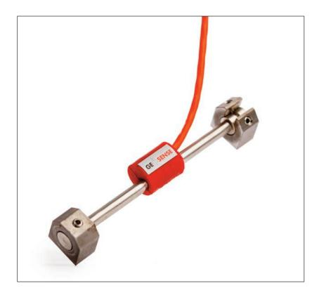
Geosense® VWS-2000 series vibrating wire surface strain mount gauges are designed for the long term monitoring of steel or concrete structures. Gauges may be attached to steel structures by arc welding or, using alternative end blocks, bonded or grouted into concrete.
