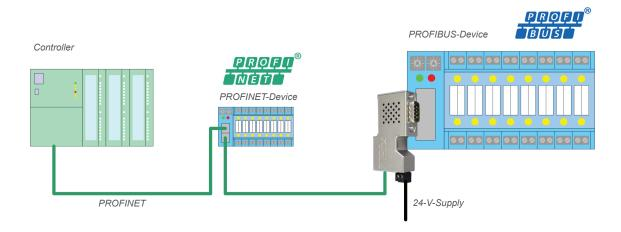
netLINK PROXY is plugged directly onto the PROFIBUS-DP connector of the slave. It is powered by 24 V. The RJ45 PROFINET jack is to be connected to PROFINET. The PROXY is configured via a PC with the configuration tool suite SYCON.net.
