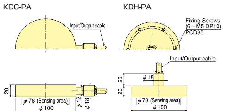
The KDG-PA and KDH-PA are stainless-steel soil pressure gauges each 100 mm in outside diameter. They are load-cell-type soil pressure gauges and designed with a high level of resistance to lateral pressure. The difference between these two models is the way the cable is attached to the gauge body.
