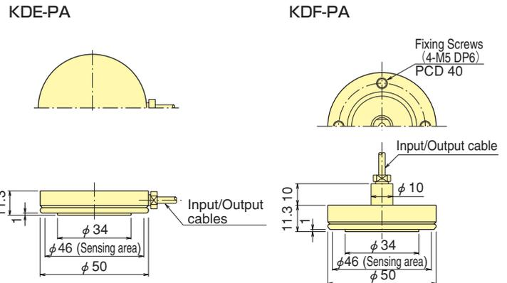
The KDE-PA and KDF-PA are soil pressure gauges each 50 mm in outside diameter. They are small in size and have a dual diaphragm structure, so they are widely used to conduct model experiments. With the KDE-PA, the Input/Output cable comes from the side of body, while with the KDF-PA, it comes from the center of the back of body. This is the difference between these two models.
