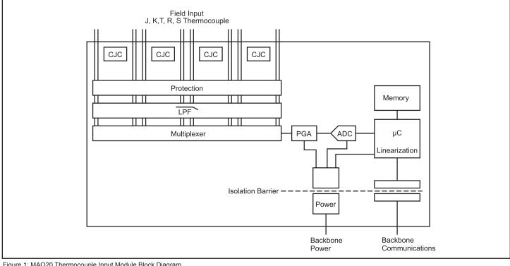
Figure 1: MAQ20 Thermocouple Input Module Block Diagram
