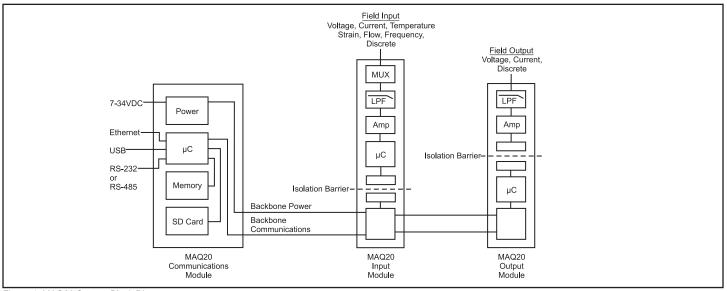
Figure 1: MAQ20 System Block Diagram
