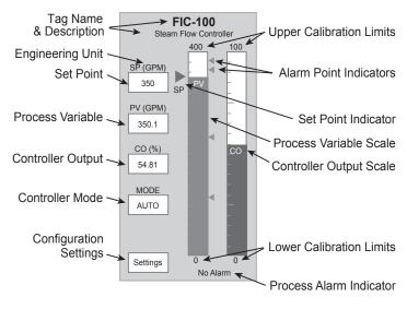
Figure 5: PID Faceplate in ReDAQ Shape Software
