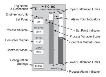
Figure 2: PID Faceplate in ReDAQ Shape Software
