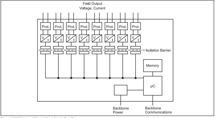
Figure 1: MAQ20 Voltage & Current Output Module Block Diagram
