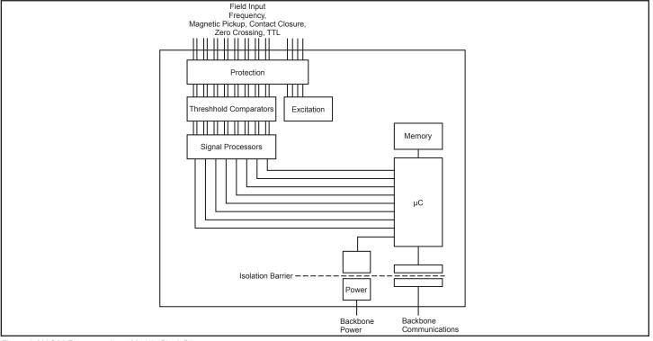
Figure 1: MAQ20 Frequency Input Module Block Diagram
