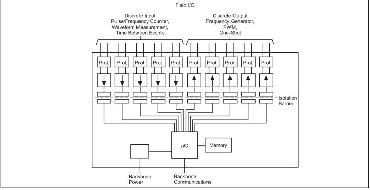
Figure 1: MAQ20-DIOL Discrete Input/Output Module Block Diagram
