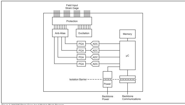
Figure 1: MAQ20 Strain Gage Input Module Block Diagram
