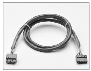
Figure 2: Backbone Expansion Cable
