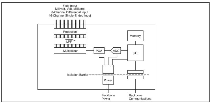
Figure 1: MAQ20 Voltage & Current Input Module Block Diagram
