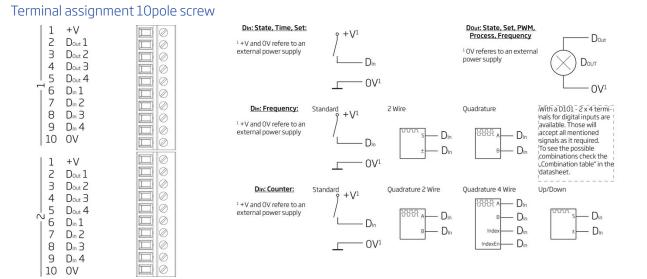
TTL and HTL-Logic voltages can be switched in the module settings via software
