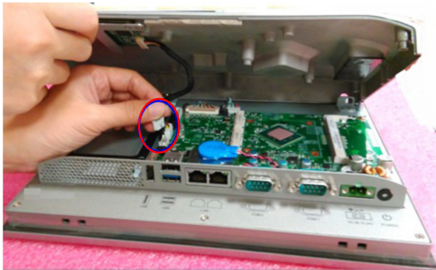
Figure 2.5 Disconnect E-Eye display cable from the main board
