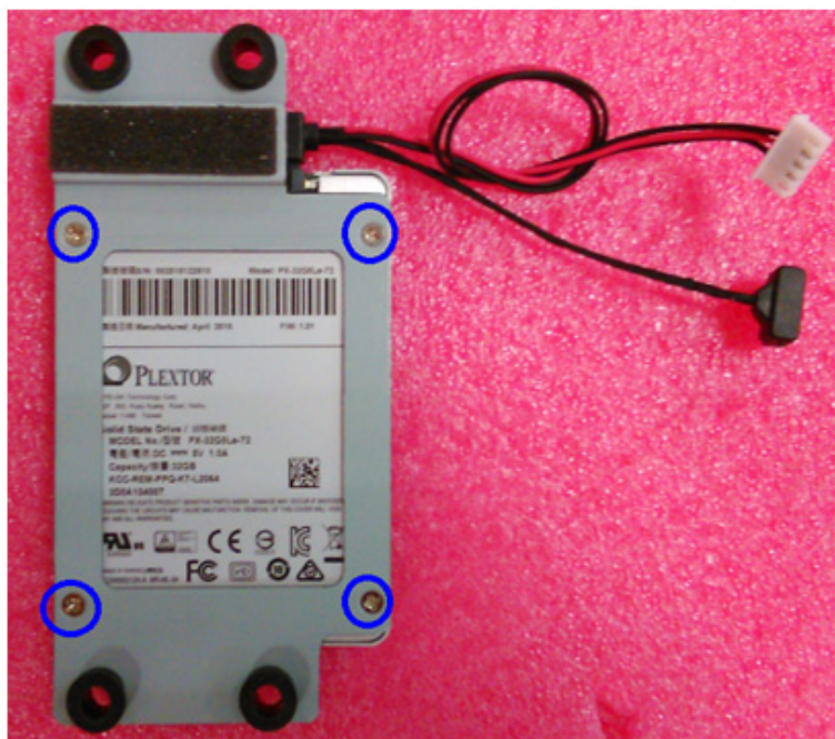
Figure 2.11 Secure SATA HDD with screws
