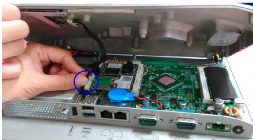
Figure 2.20 Replacing the rear cover
