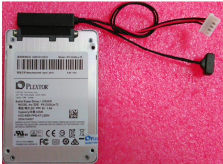
Figure 2.10 SATA cable connected to SATA HDD
