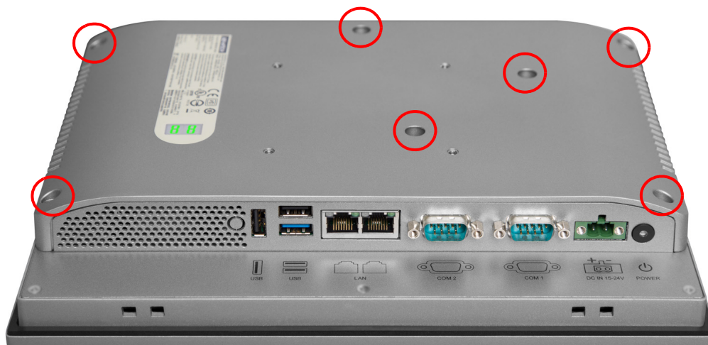
Figure 2.4 Retention screws on rear cover
