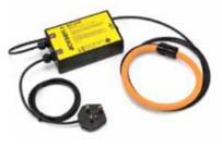
All Electrocorders sample every input 16 times per cycle, a cycle is 20ms at 50Hz or 16ms at 60Hz.
