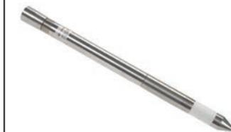
Geosense® VWP-3000 Series of Vibrating Wire piezometers use the well-proven method of converting fluid pressures on a sensitive diaphragm into a frequency signal.
